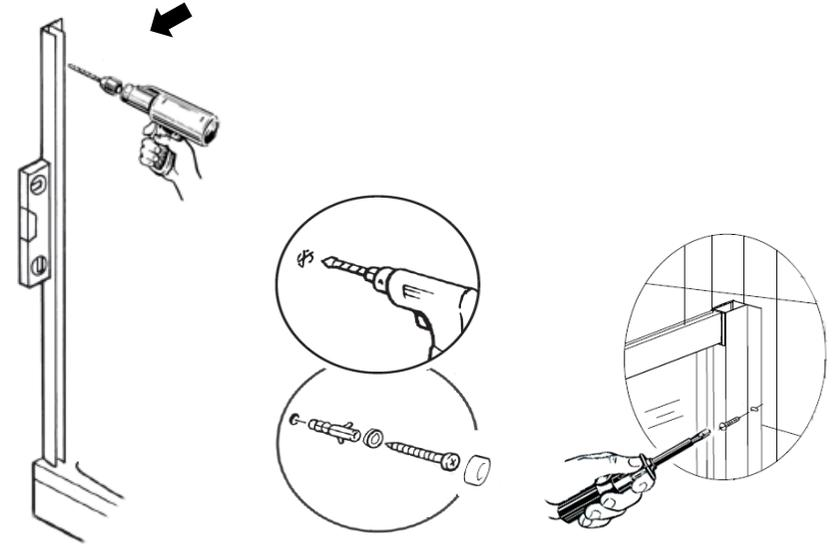
After drilling, insert wall plugs and tap in so flush with finished wall.
